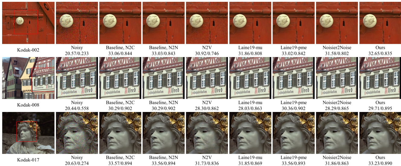
Figure A.2: Visual comparison of our method against other competing methods in the setting of Gaussian \sigma = 25 . The quantitative PSNR(dB)/SSIM results are listed underneath the images. Best viewed in color.
