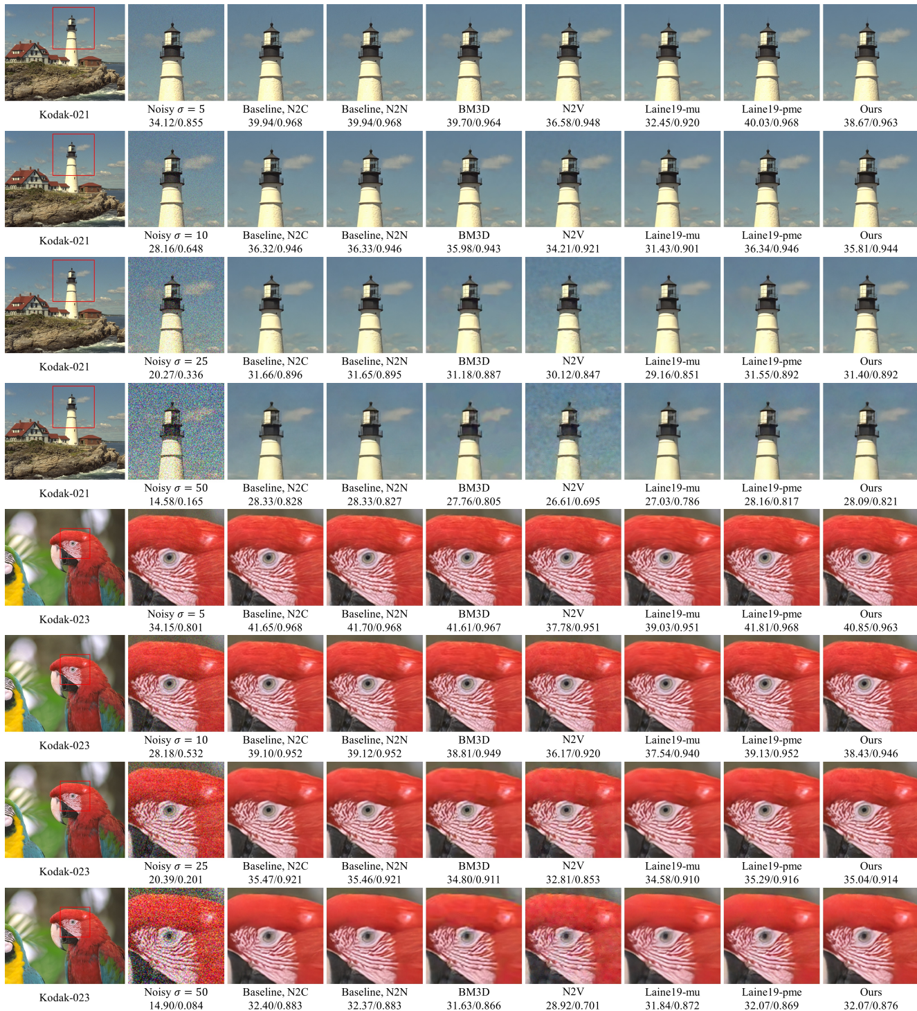
Figure A.4: Visual comparison of our method against other competing methods in the setting of Gaussian \sigma \in [5, 50] . The denoised results of four noisy images with fixed Gaussian noise level \sigma = 5, 10, 25, 50 are evaluated on the same denoising model which is trained on noisy images with Gaussian \sigma \in [5, 50] . The quantitative PSNR(dB)/SSIM results are listed underneath the images. Best viewed in color.
