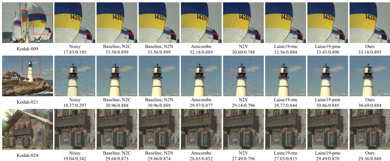
Figure A.3: Visual comparison of our method against other competing methods in the setting of Poisson \lambda = 30 . The quantitative PSNR(dB)/SSIM results are listed underneath the images. Best viewed in color.
